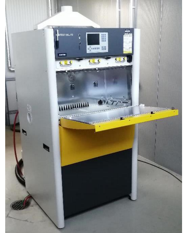
Weathering system at JKI: UV-Suntest XXL (Atlas)
