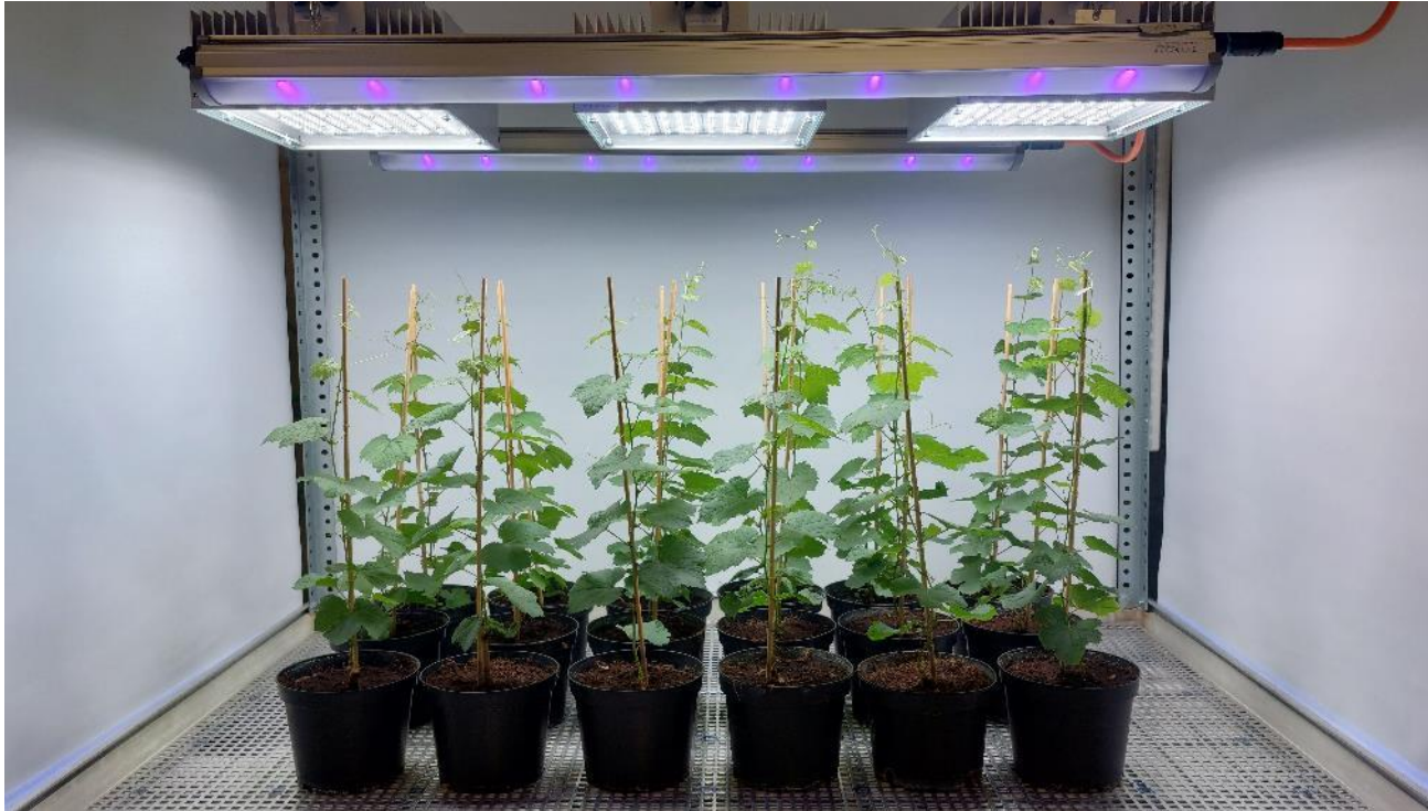
Radiation test system at Hochschule Geisenheim: LED-KE 400 VSP + LED-MID UV-A
